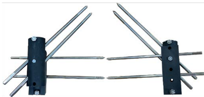
Figure 5. Lateral side and medial side of the external fixator prototype with inserted screws.
